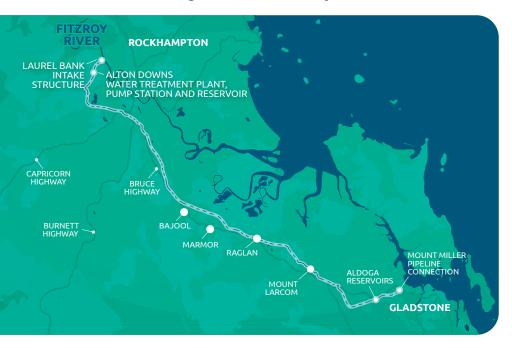
The 117-kilometre pipeline will run from the Lower Fitzroy River in Rockhampton and connect to Gladstone Area Water Board's existing water network at Yarwun. The pipeline comprises a water treatment plant, reservoirs and pumping stations at locations along its alignment including Laurel Bank, Alton Downs and Aldoga.
