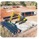
The brand new SafeVac SV400 model from Austrack Equipment Pty Ltd can safely lift and manoeuvre the mild steel cement lined pipes from the trucks into the laydown site. The SafeVac SV400 was designed and manufactured locally in Queensland and a few of its impressive features include:
