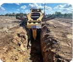
trenchers have a large, toothed metal wheel on the front that can cut through soil at varying depths, while simultaneously pushing excavated materials to the side using spacers and ejectors.
