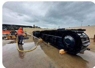
Tracks frames of the Trencher T1660 Magnum being washed at the Port of Gladstone.
