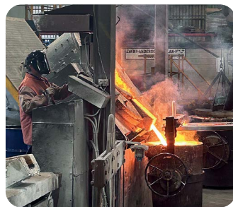
An isolation valve being cast at the White's Foundry facility.
